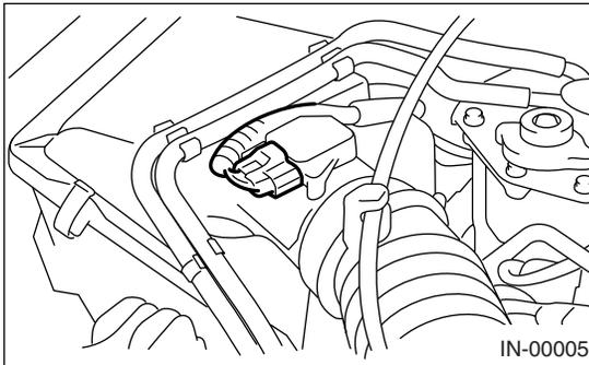
3) Loosen the clamp (A) which connects air intake boot and intake duct.
