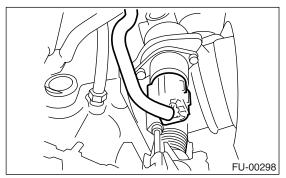
3) Remove the idle air control solenoid valve from the throttle body.
