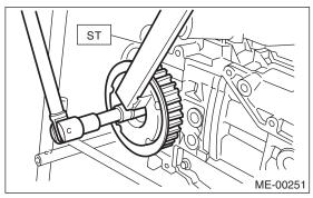
2) Install the cam sprocket No. 2. To lock camshaft, use ST.
