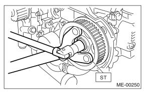
7) Remove the cam sprocket No. 1. To lock the camshaft, use ST.
