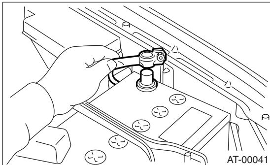
2) Remove the lower cover and then disconnect the connector.
