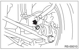
3) Remove the bolt which secure stabilizer to stabilizer bracket.
