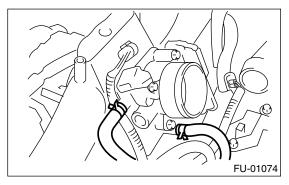
5) Remove the bolts which secure the throttle body to intake manifold.
