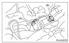
4) Disconnect the engine coolant hoses from the throttle body.
