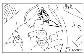
5) Remove the engine coolant temperature sensor.
