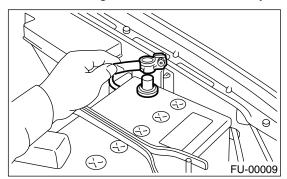
2) Disconnect the connectors from manifold absolute pressure sensor.
