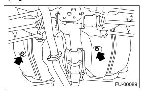
6) Tighten the fuel drain plug.
