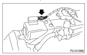
4) Remove the bolt which installs the fuel level sensor on mounting bracket.
