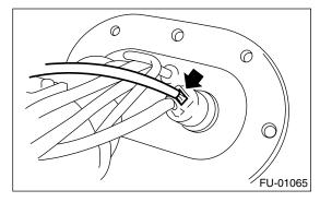
3) Remove the fuel temperature sensor.
