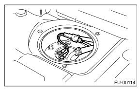
9) Remove the bolts which install the fuel sub level sensor on fuel tank.
