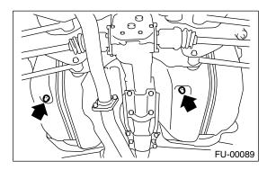
4) Tighten the fuel drain plug.
