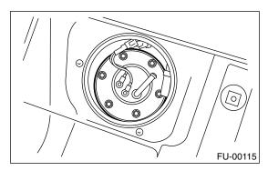
10) Remove the fuel sub level sensor.
