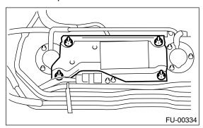
3) Move the clip and disconnect the evaporation hose from fuel cut valve.
