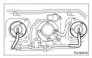
4) Remove the bolts which install the fuel cut valve.
