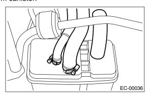
3) Remove the canister from body.
