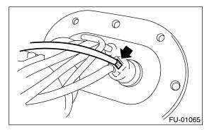
3) Remove the main fuel level sensor from fuel pump assembly. <Ref. to FU(STi)-57, REMOVAL, Fuel Level Sensor.>
