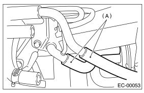
6) Remove the bolt which installs the drain filter and drain valve brackets on body, and remove them as a unit.
