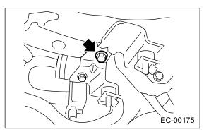
7) Disconnect the evaporation hoses, and remove the drain filter from the bracket.
