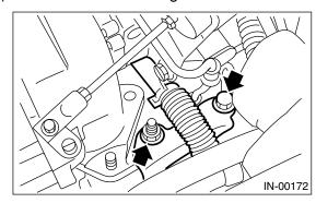
12) Disconnect the oil outlet hose from pipe.
