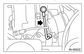
4) Install the joint pipe to turbocharger.
