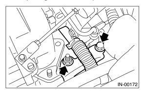
7) Connect the engine coolant hose which is connected to coolant filler tank.
