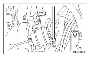
3) Install the oil pipe to turbocharger.
