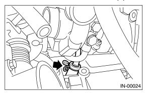
2) Install the turbocharger to intake duct.
