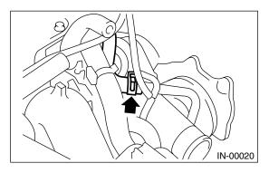
7) Loosen the clamp which secures the turbocharger to intake duct.
