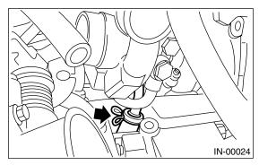
13) Take out the turbocharger from engine compartment.
