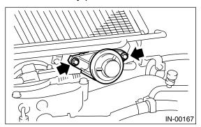
2) Disconnect the air by-pass hoses from air by-pass valve.
