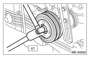
3) Remove the crankshaft pulley.
