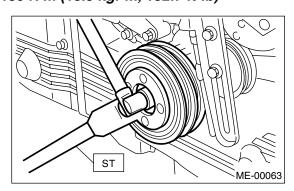
3) Confirm that the tightening angle of crankshaft pulley bolt is 65 degrees or more. If the tightening angle of crankshaft pulley bolt is less than 65 degrees, conduct the following procedures.
