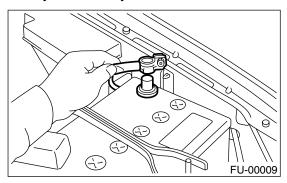
2) Disconnect the washer motor connector.
