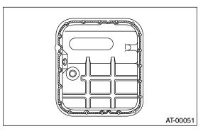
5) Apply liquid gasket fully to three holes other than screw holes on transmission case.
