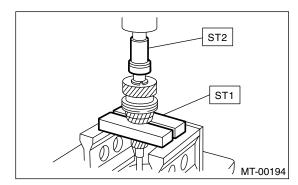
6) Using the ST1 and ST2, install the 5th gear thrust washer and 5th needle bearing race onto the rear section of transmission main shaft.
