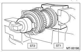
3) Remove the 5th-Rev sleeve and hub assembly, baulk ring, 5th drive gear and needle bearing.
