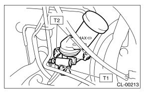
2) Connect the push rod of master cylinder to clutch pedal, and install the clevis pin and snap pin.
