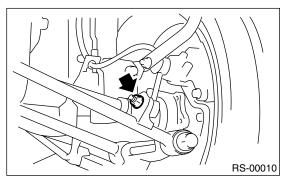
3) Remove the bolt and nut which secure the stabilizer to stabilizer bracket.
