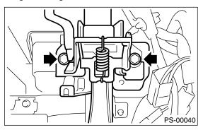
10) Pull out the steering shaft assembly from hole on toe board.
