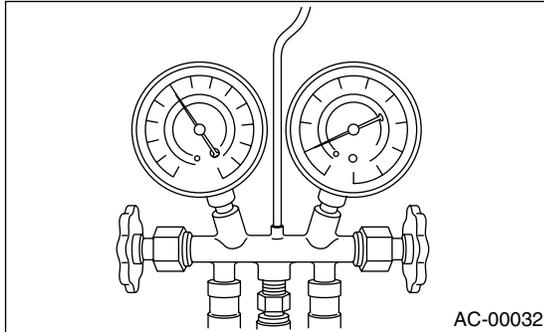
19) If the HFC-134a source is empty, close the high-pressure valve, close the valve on the can tap, and replace the HFC-134a source with a new one to restart the operation.
