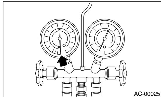
6) After 15 minutes of evacuation, if the reading shows 100.0 kPa (750 mmHg, 29.5 inHg) or higher, close the valves on the both sides to stop the vacuum pump.
