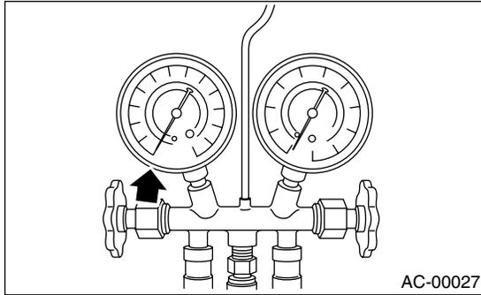
8) Leave it at least 5 minutes, and then check the low-pressure gauge reading for any changes. When a gauge indicator shows near to zero point, this is a sign of leakage. Check pipe connector points, repair them, make sure there is no leakage by air bleeding.
