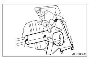
3) Remove the heater core.
