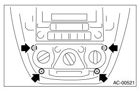
7) Pull out the control unit and disconnect connectors.
