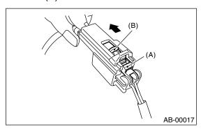
(3) With the slide lock (B) pulled, remove the lock arm (A) to its original position, and then pull in the direction of the arrow and separate the connector.
