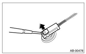
(2) Pull the connector to disconnect from driver's side airbag module assembly or retractor assembly.
