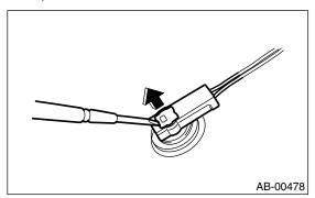
(2) Pull the connector to disconnect from retractor assembly.
