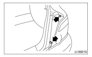
3) Remove two bolts, and then remove the rear combination light while disconnecting connector.
