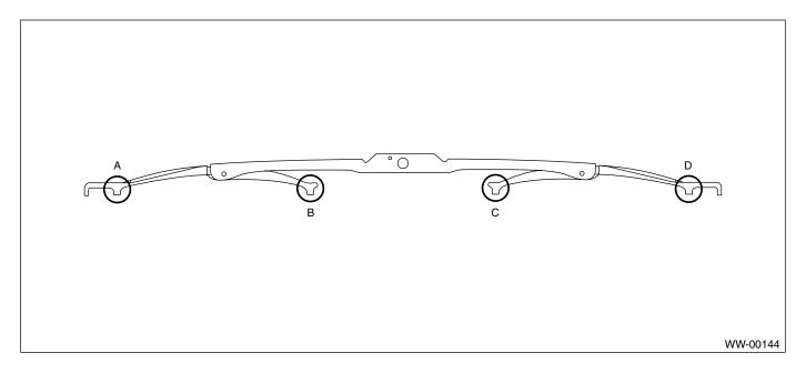
1) Insert the wiper rubber through the claw (B).
