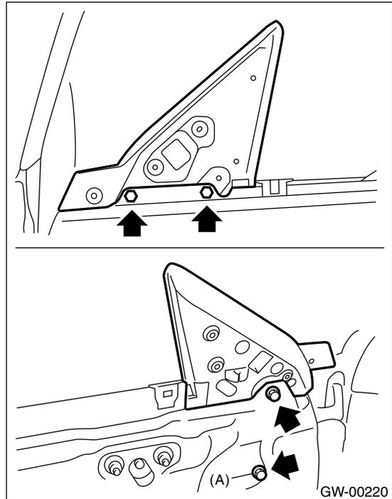
14) After adjustment, tighten the bolts and nuts.
