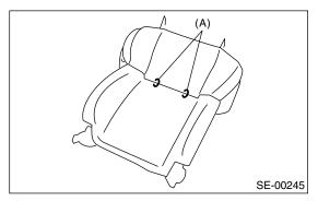
13) Remove the connecting wire (A), and then loosen the bolts and nuts to remove slide rail.
