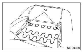
8) Remove the hog rings (A) at side of inside backrest from backrest frame.
