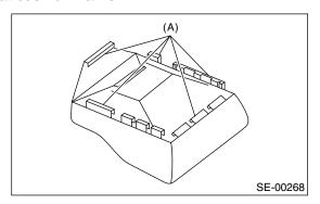
16) Remove the hog rings (A), and then remove the seat cushion cover from seat cushion pad.
