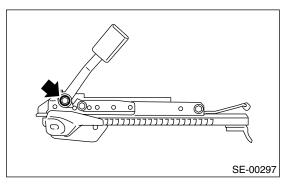
15) Remove the hook (A), and then remove the seat cushion frame.
