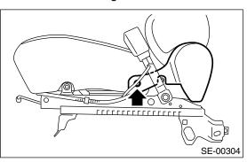
4) Remove two bolts from reclining hinge on each side.
