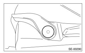
3) Remove the reclining lever and seat hinge outer cover.
