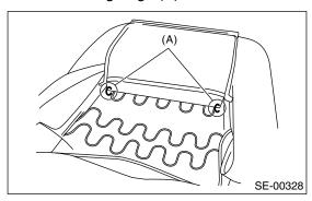
9) Remove the hog rings (A) which secure the backrest cover and backrest pad.
