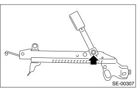
14) Remove the hooks (A), and then remove the seat cushion frame.
