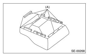
15) Remove the hog rings (A), and then remove the seat cushion cover from seat cushion pad.
