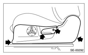
4) Remove the seat hinge inner cover.
