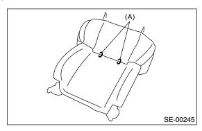
12) Loosen the bolts and nuts to remove the seat cushion from slide rail.
