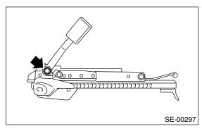
15) Remove the hook (A), and then remove the seat cushion frame.
