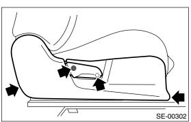
3) Remove the seat hinge inner cover.
