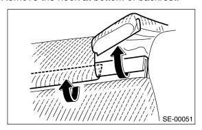
7) Open the zipper behind of backrest. (Side airbag equipped seat)
