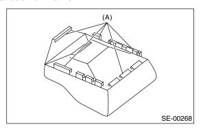
15) Remove the hog rings (A), and then remove seat cushion cover from seat cushion pad.
