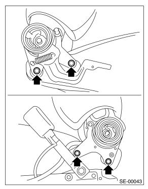
5) Remove the hook at bottom of backrest.
