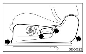
4) Remove the seat hinge inner cover.
