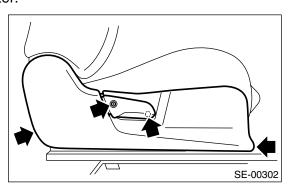
3) Remove the seat hinge cover inner.
