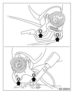
6) Remove the hook at bottom of backrest.
