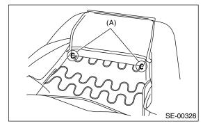
8) Remove the hog rings (A) which secure the backrest cover and backrest pad.
