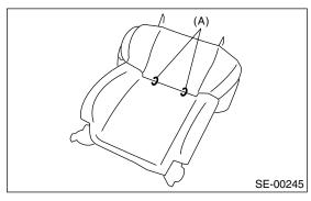
13) Remove the connection wire (A), and then loosen the bolts and nuts to remove slide rail.
