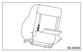
8) Remove the hog rings (A) of backrest cover. (Side airbag equipped seat)
