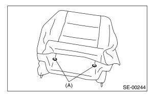
12) Remove the hog rings (A) at front of seat back, and then remove the seat back cover from seat back.
