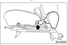
4) Remove the bolts from reclining hinge on each side.
