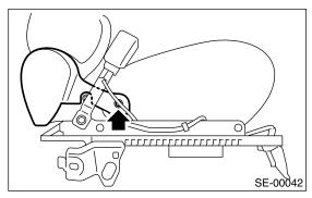
5) Remove two bolts from reclining hinge on each side.
