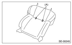
12) Loosen bolts and nuts to remove the seat cushion from slide rail.
