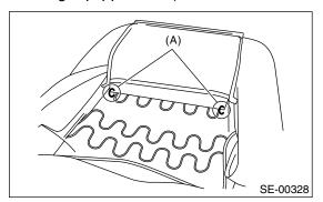
9) Open the zipper behind of backrest cover, and then remove the hog rings (A) at side of inside backrest from backrest frame.
