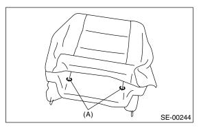
11) Remove the hog rings (A) at front of seat back, and then remove the seat back cover from seat back.
