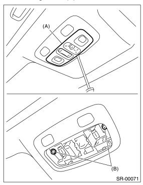
3) Disconnect the harness connectors and remove the sunroof switch.
