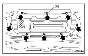
6) Install the hood insulator with new clips.
