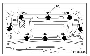
3) Loosen the six nuts (B), remove the four clips (A), and then remove the hood grille.
