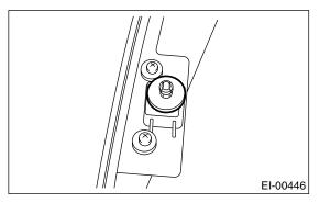
2) Engage the four clips of hood grille to front hood panel.
