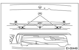
5) Install the hood duct with clip (A) and seven bolts.
