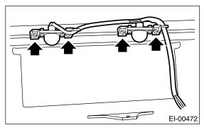
14) Remove the six clips, and then remove the bumper side cover.
