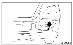
11) Remove the three bolts, then remove the bumper beam.
