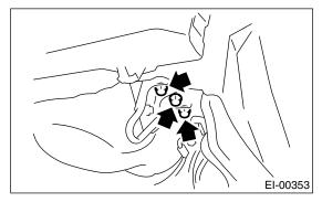
12) Remove the five clips, and then remove the bumper upper beam.
