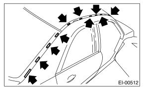
2) Put the front edge of roof molding onto front window molding, and insert the front locating pin into body side cap.
