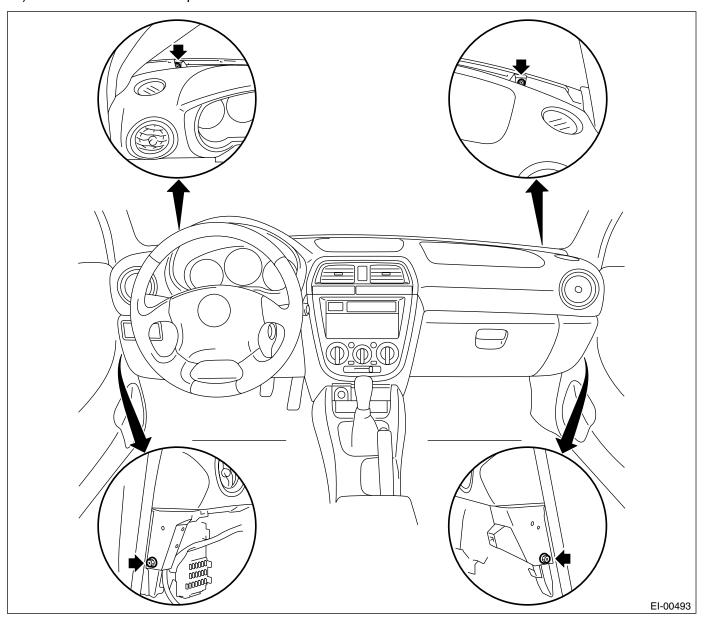
12) Check that all the harness is disconnected, and then remove the instrument panel from vehicle.
