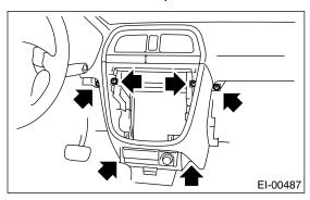
8) Remove the hook, and then remove the defroster panel.
