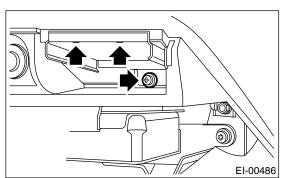
7) Loosen the four screws and two nuts, and then remove the lower console panel.
