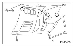
3) Remove the clip (A), and then remove the center console panel.
