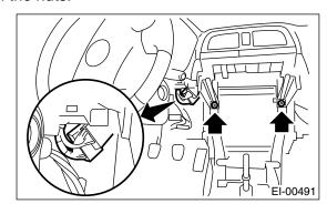
11) Remove the instrument panel installation bolts.
