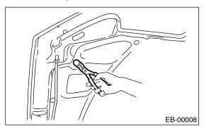
3) Remove the bolts to remove the front hood from hinges.
