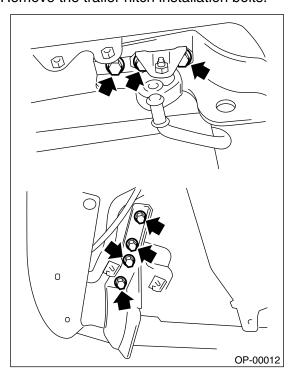
5) Remove the trailer hitch while lowering exhaust pipe.
