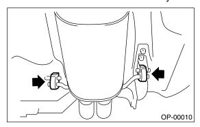
3) Remove the three nuts and canister.
