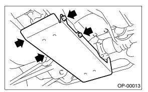
3) Loosen the nuts until the rear differential protector can be removed.
