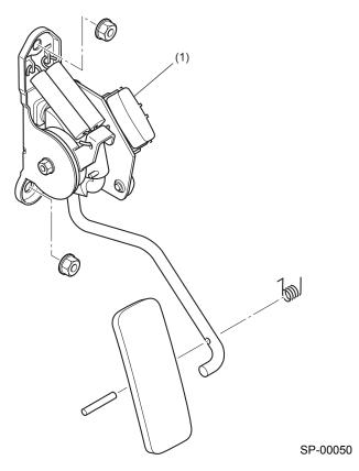
(1) Accelerator pedal position sensor
