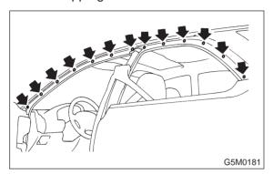
3) Installation is in the reverse order of removal.NOTE:Insert clips onto hooks, then fasten with screws.
