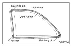
(3) Stick them fast by pressing all sides lightly.7) Water leakage test:
