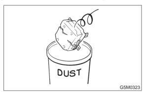
• After removal, keep the airbag control module on a dry, clean surface away from heat and light sources, and moisture and dust.
