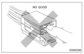
• When cpnnecting or disconnecting airbag connector, make sure ignition switch is OFF.
