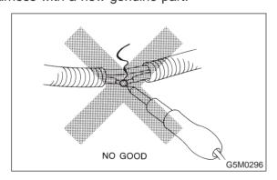
• Install the wire harness securely with the specified clips so as to avoid interference or jamming with other parts.
