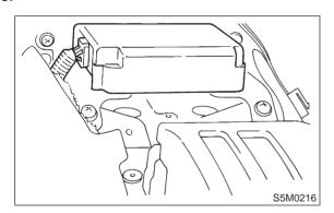
7) Disconnect body harness connector (B31) from connector (AB1).
