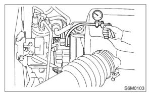
3) Make sure that cruise control cable moves smoothly and quickly when a vacuum pressure of 40.0 kPa (300 mmHg, 11.81 inHg) is applied to actuator.
