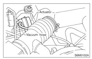
2) Connect vacuum pump as shown in figure.
