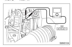
: Is resistance less than 69  $\Omega$ ? (CHECK)
