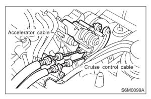
installed to the left of the accelerator cable?
