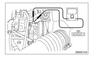
CHECK) : Is resistance less than 100  $\Omega$ ?
