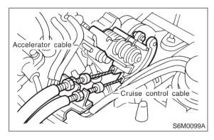
CHECK : Does the accelerator cable throttle cam move when the cruise control throttle is moved by hand?
