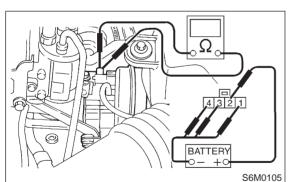
CHECK : Does cruise control cable have a stroke of 35 mm (1.38 in) within 3 sec-
