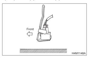
CHECK : Is the voltage between 0.5 and 0.9 V when G sensor is inclined backwards to 90°?
