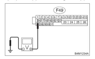
(CHECK): Is the voltage between 10 V and 17 V?
