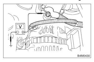
CHECK : Is the voltage between 10 V and 17 V?
