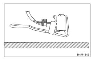
CHECK : Is the voltage between 2.1 and 2.5 V when G sensor is horizontal?
