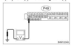
: Is the voltage between 10 V and 15 V? CHECK
