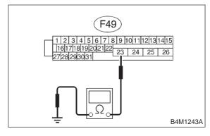
$\widehat{\text{CHECK}}$ : Is the resistance less than 0.5  $\Omega$ ?
