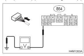
CHECK): Is the voltage between 10 V and 15 V?
