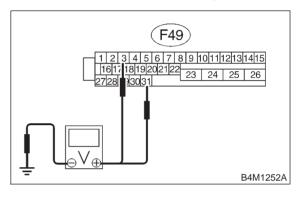
CHECK): Is the voltage between 10 V and 15 V?
