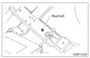
8) Use engine grounding terminal or engine proper as the grounding point to the body when measuring voltage and resistance in the engine compartment.
